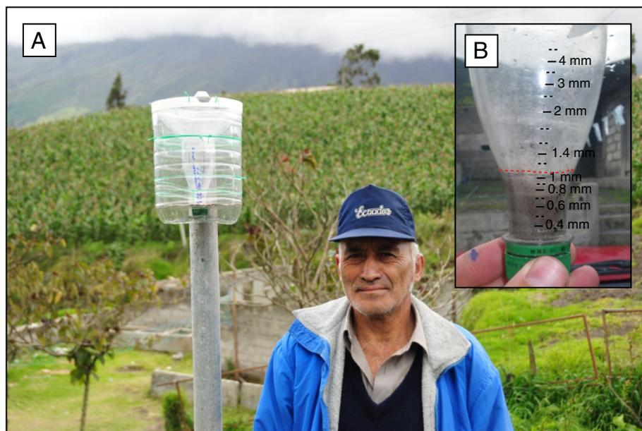
**Figure 5** Installation of an ashmeter and sampling. **A**) Example of an ashmeter deployed in the backyard of Rodrigo Ruiz on January 14, 2012 (Pillate); **B**) An example of a thin (1.1 mm-thick) deposit collected March 14, 2012 in Pillate, from the February 4, 2012 eruption.
