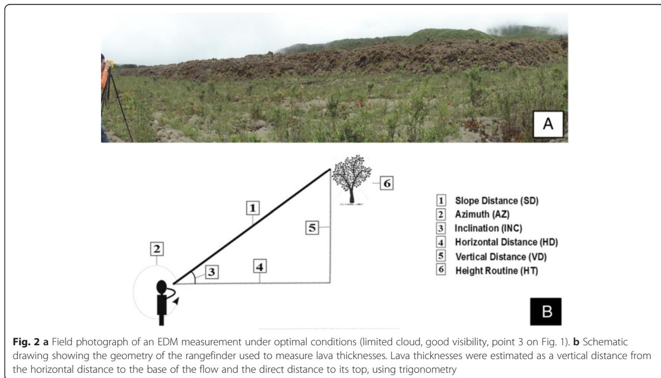
**Fig. 2 a** Field photograph of an EDM measurement under optimal conditions (limited cloud, good visibility, point 3 on Fig. 1). **b** Schematic drawing showing the geometry of the rangefinder used to measure lava thicknesses. Lava thicknesses were estimated as a vertical distance from the horizontal distance to the base of the flow and the direct distance to its top, using trigonometry
